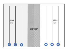
Due to spacing in the special field rules, you have a 660' corridor going down the middle of the two units. You have both units under lease, and you have the ability to obtain an Allocation Well permit. Your idea is to drill something like this:
