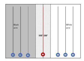
The Lease Line Allocation Well pictured above is great in theory and looks clean on a permit map. It is a straight line. However, I used to work in directional drilling and can attest that there is no such thing as a straight line in drilling wells. Rather, the as-drilled plat is usually something that looks like this:
